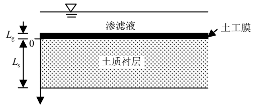
图 1 有机污染物在复合衬层中一维扩散示意图 Fig.1 Sketch of organic contaminants diffusion through composite liners
